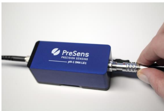
Fig. 3 Connecting the temperature sensor
