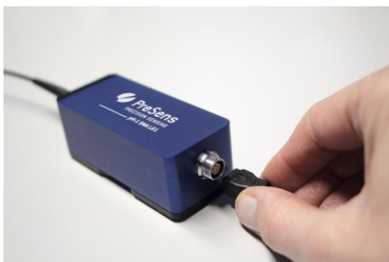
Fig. 2 Connecting the USB cable
